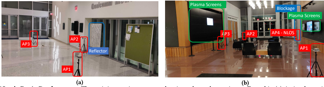
Figure 8: DLoc’s Basic Deployment: The training environment and train and test data points collected in (a) A simple environment that spans 500 sq. ft. space with 4 access point.(b) A complex environment that spans 1500 sq. ft. space with 4 access points.
